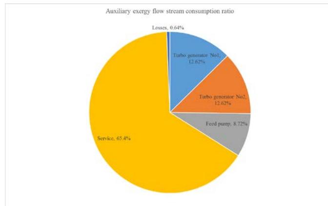
Fig.6. Exergy ratio of auxiliary requirements for marine plant at propulsion shaft speed of 25.52 min<sup>-1</sup>
