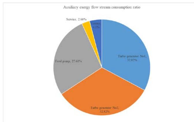
Fig.7. Exergy ratio of auxiliary requirements for marine plant at propulsion shaft speed of 83 min<sup>-1</sup>
