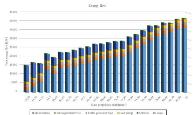
**Fig.3. Exergy flow rates under main propulsion shaft speed variation**
