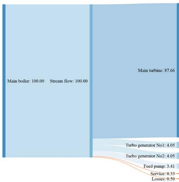
Fig.5. The exergy ratio in (%) at 83 min<sup>-1</sup> of the main propulsion shaft
