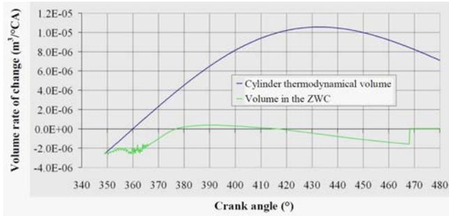
Fig.3. Thermodynamic volume rate of change in the cylinder and in the ZWC
