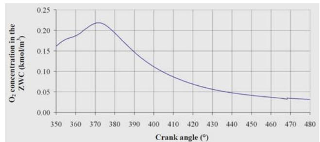
Fig.7. The equilibrium molar concentration of O<sub>2</sub> in the zone without combustion
