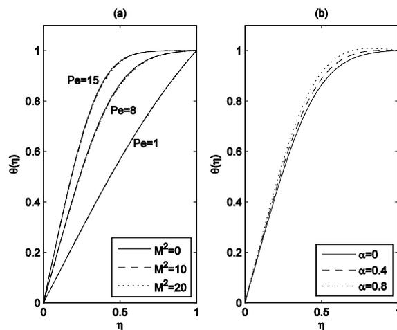
Fig. 5 (a) Temperature profiles for  $\alpha = 0$ , (b) Temperature profiles for  $Pe = 8$  and  $M^2 = 1$
