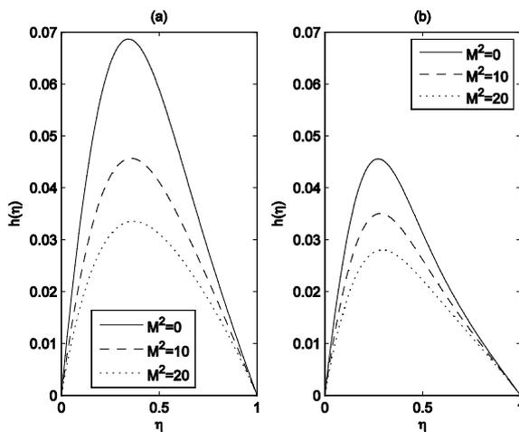
Fig. 4 (a) Axial velocity profiles for  $R = 10$ , (b) Axial velocity profiles for  $R = 20$
