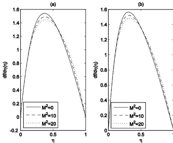
Fig. 3 (a) Tangential velocity profiles for  $R = 10$ , (b) Tangential velocity profiles for  $R = 20$
