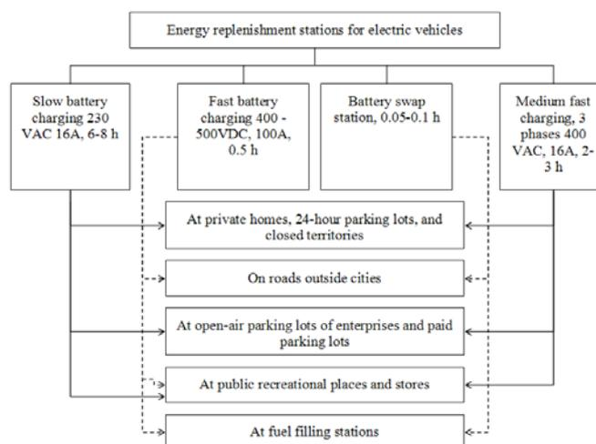
Fig.1. Energy replenishment stations for electric vehicles
