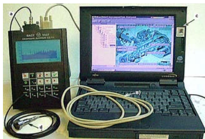
Figure 2. Vibration portable set on the vibration analyzer CD-12M base, produced by company BACT (Russia) [2]
