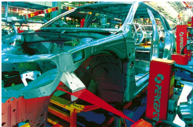
Fig.11 Laser control of car body on line
