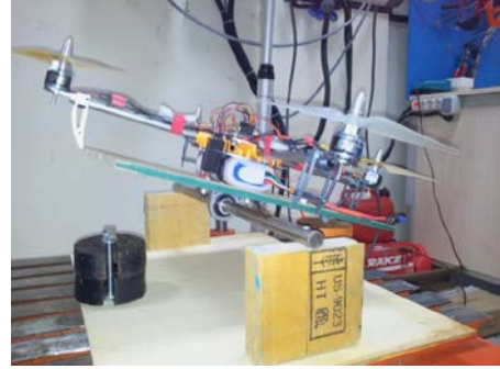
Picture 3: 3DOF Test platform for quadcopter, multicopter and helicopter around ball bearing fixture
