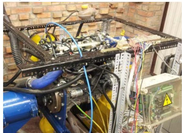
Fig. 2.1. 1.3 JTD 16V engine on the test bed.
