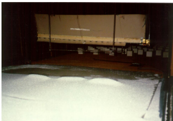
Fig. 13 Snow deposits determined by the presence of barriers
