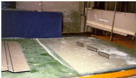
Fig. 11 Model of the road with a protection barrier of snow fences
