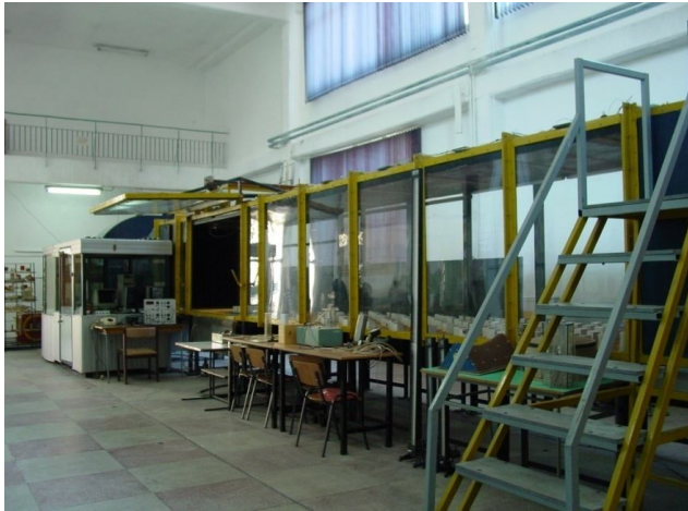
Fig. 5 Wind tunnel SECO 2 in the Laboratory of Structural Aerodynamics of the Faculty of Constructions and Building Services in Iași
