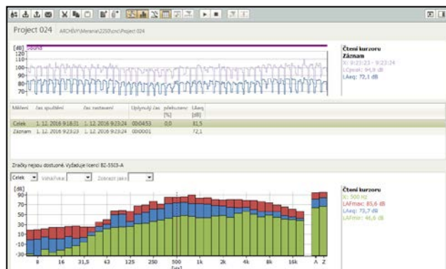
Fig. 7: Record of measurement of noise level A exposure at 500 Hz
