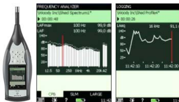
Fig. 3: Hand- held Analyzer Type 2250, module for frequency analysis and time module
