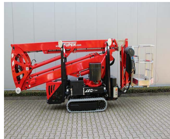
Fig. 6 Platform on its own belted chassis [3]
