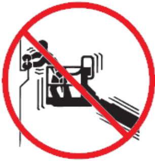
Fig. 14 Prohibition on pulling/pushing objects outside the platform [6]
