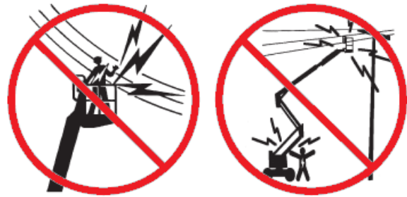
Fig. 11 Prohibition on nearing power lines [6]
