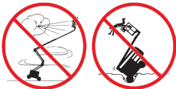
Fig. 13 Prohibition on operating in strong wind and prohibition on moving through unsuitable terrain [6]
