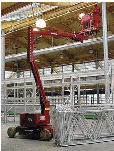
Fig. 3 Articulated platform lift on its own wheeled chassis [2]
