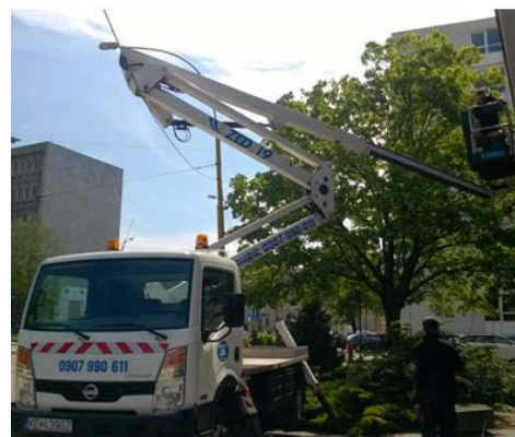
Fig. 5 Articulated – telescoping platform lift on an automobile chassis
