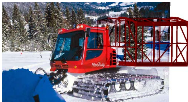
Fig. 1 Snow groomer Piston Bully 200 with the model of the passenger cabin
