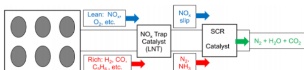
Fig. 5 Coupled LNT-SCR System for NO_x reduction [15].
