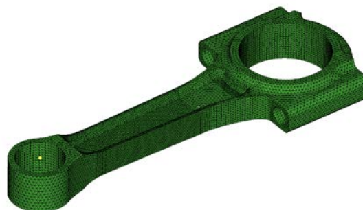
Fig.2 : Mesh in connecting rod.
