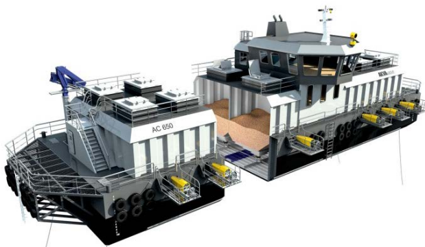
Fig. 1. Fish-feeding barge (a) and its cross-section in silos bunker (b) [1, 2].
