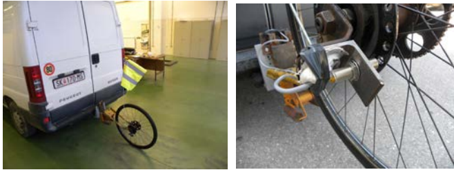
Fig. 3 Fifth wheel and a sensor for velocity measurement
