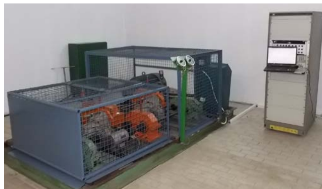
Figure 11. Transmission test bench with safety cover
