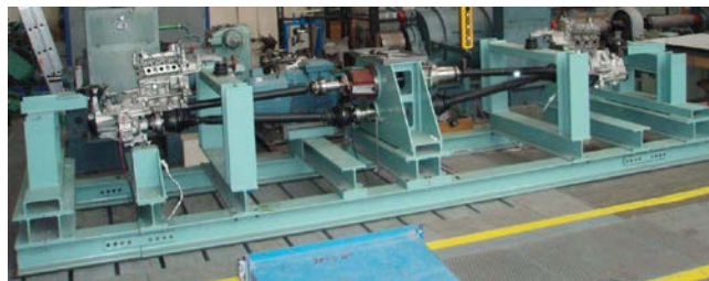
Figure 2. Test bench for testing of gearboxes (Czech Technical University in Prague)
