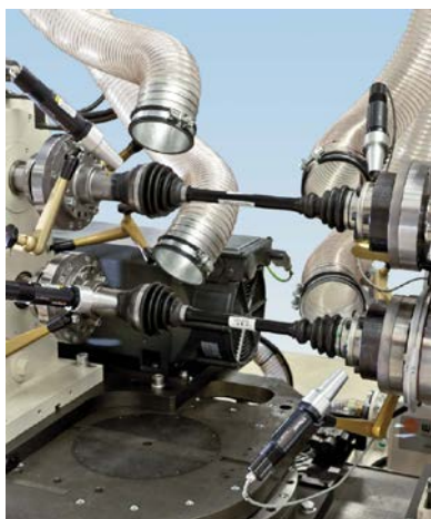
Figure 3. Test bench for testing of the articulated shaft
