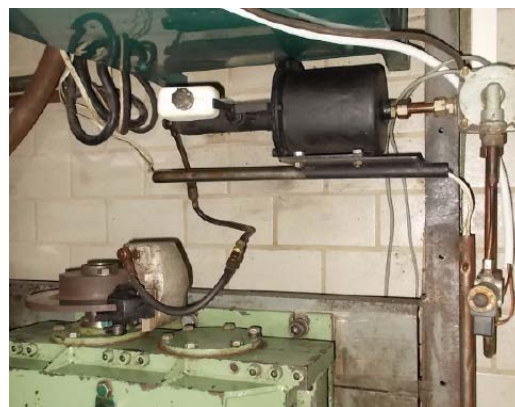
Figure 5. Braking system of the articulated half-shafts
