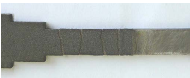
Fig. 4. Multiple cracking of the plasma-sprayed coating with thickness of 150 μm after testing of the tensile specimen. There are a lot of transverse cracks
