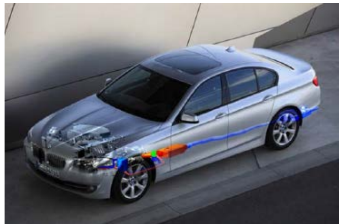
Fig. 2 BMW adds Steam Engine to improve fuel efficiency [8].
