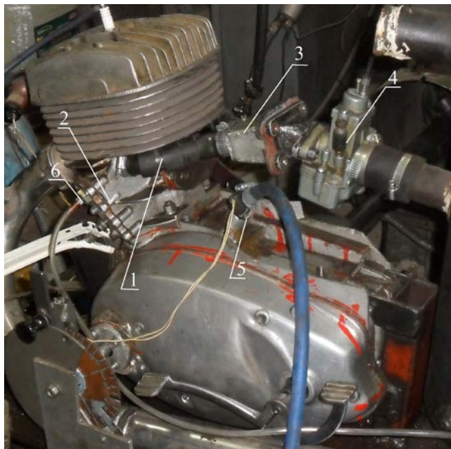
Fig. 6. Two-stroke engine with stratified mixture formation and injection gasoline
