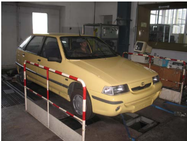
Fig. 2 Investigations of vehicles on rolls
