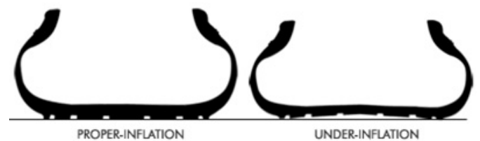
Fig. 9. The reduced pressure tyre exerts on the road surface when tires are under-inflated
