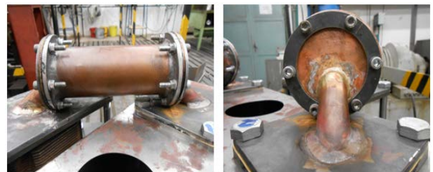
Fig. 6 Real model of the regenerator.
