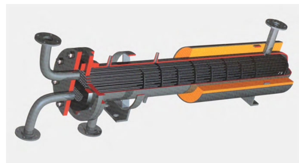
Fig. 5 Shell & tube heat exchanger
