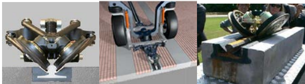
Fig. 6 The trolley's guidance.
