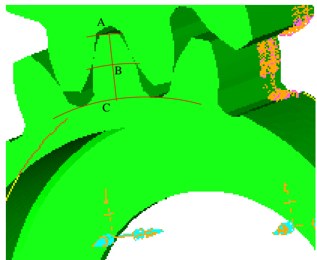
Fig.1. 3D FEM model (one half) of a solid pinion and thin-rimmed wheel engaged at the outer point of single pair tooth contact; the points A, B, C along the tooth height share about 70% and the gear teeth share only about 30%.
