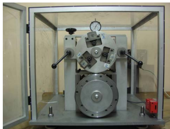
Fig. 1 Impact sliding tribotester
