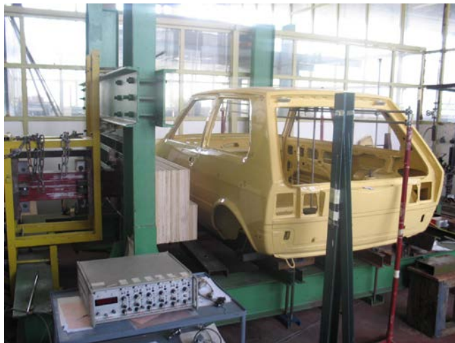
Fig. 6 Quasi-static trial according to ECE 95
