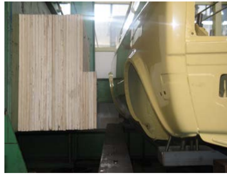
Fig. 7 Reconstructed barrier according to ECE 95
