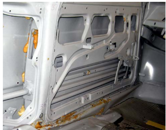
Fig. 13 Total deformation of left side door
