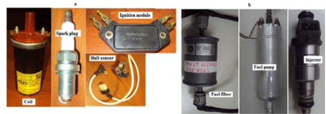
Figure 9. Components of chosen ignition (a) and injection (b) systems
