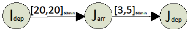
Fig. 6 Illustration of the modeling of a trip between a departure event I to an arrival event J, with a given running time with 20 minutes and a defined waiting time of 3 up to 5 minutes in J
