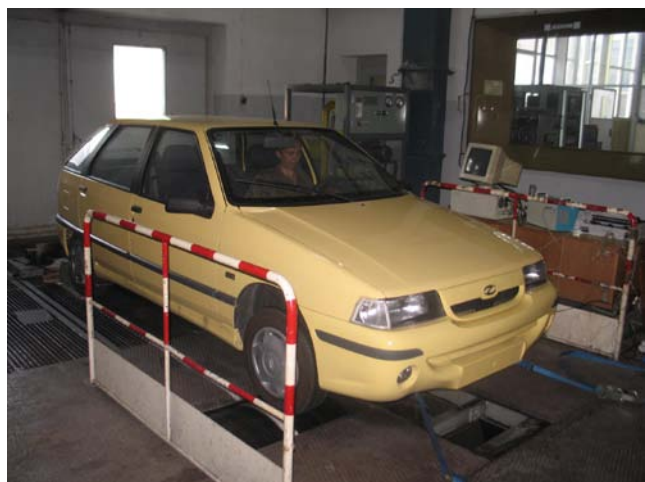
Fig. 9 Investigations of vehicles on rolls
