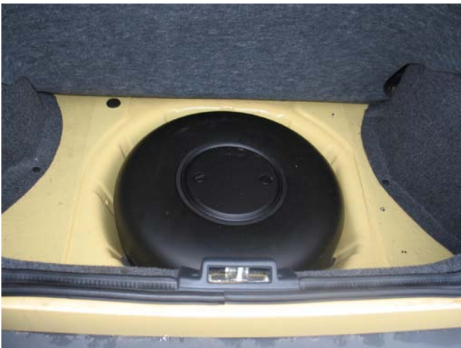
Fig. 5 Toroidal LPG tanks
