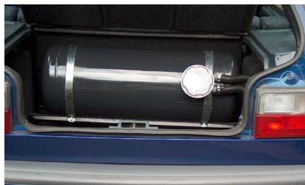
Fig. 4 Cylindrical LPG tanks
