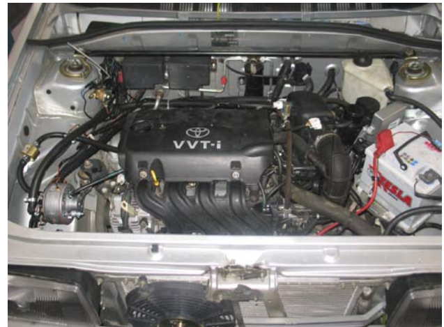
Fig. 8 Sequential systems for LPG Alisei N Zavoli
